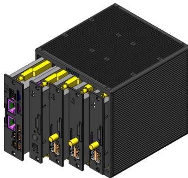
Fig. 1. UBTECH's newly developed multi-core heterogeneous processor hardware platform
