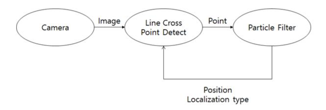
Figure 1. The S/W architecture on localization of ALICE
