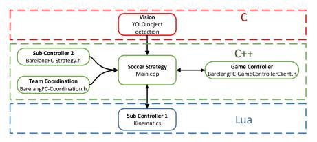
Fig. 2. Block diagram of software system.
