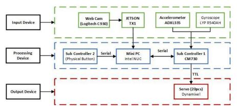
Fig. 1. Block diagram of hardware system.
