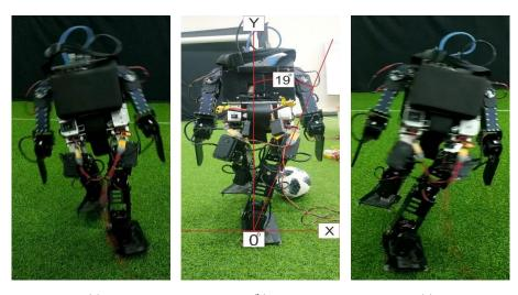
(b) (a) (c) Fig. 10. Robot behavior when side kick (a) less than  $18^{\circ}$  (b)  $19^{\circ}\pm1^{\circ}$  (c) greater than  $21^{\circ}$ .
