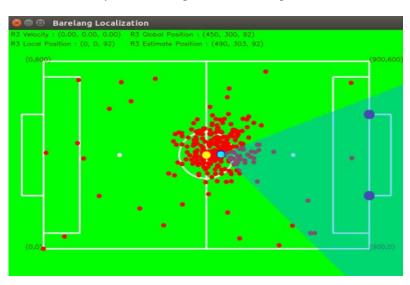
Fig. 9. Position predictions from particle filters.
