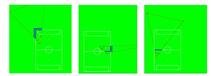
**Fig. 7.** The visibility status of observations in different positions of robot. In the right image some observations are in the polygon that describes the field of view but they are not visible due to their large distance from the robot.
