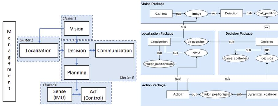
**Fig. 1.** Cross Architecture implemented. **Fig. 2.** ROS 2 architecture being implemented.
